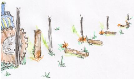
2. We mark where the intermediate posts are to go, and place the posts beside these marks. The tractor and post driver drive along the line and drive each post down.
