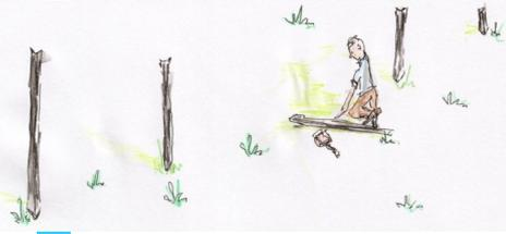
1. To construct a fence the first stage is to 'mark out' where the fence line is going. We do this by placing standards one each end with several between these, then lining them up to get a straight line.
